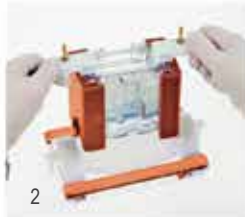
2 Transfer to casting base and tighten cams.
