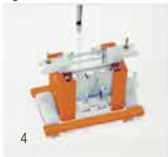
4 Pour gel solution, insert combs and allow gel to polymerize.
