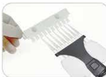
All combs are multichannel pipette compatible
