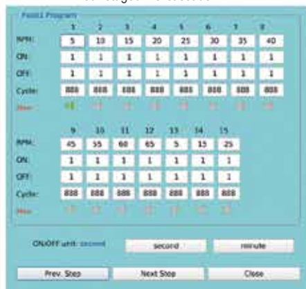
15-Step programmable PID control
