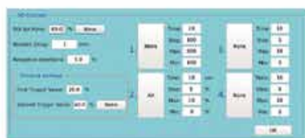
Four-staged DO cascade
